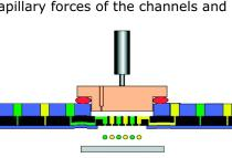
the surface tension of the fluids in the nozzles. When this happens, the printhead accelerates the fluid and the nozzle dispenses a droplet. For a better and more homogenous ejection of the droplets, the nozzles area is uniquely coated with a hydrophobic silane. This allows for a droplet ejection like shown in the picture below.
